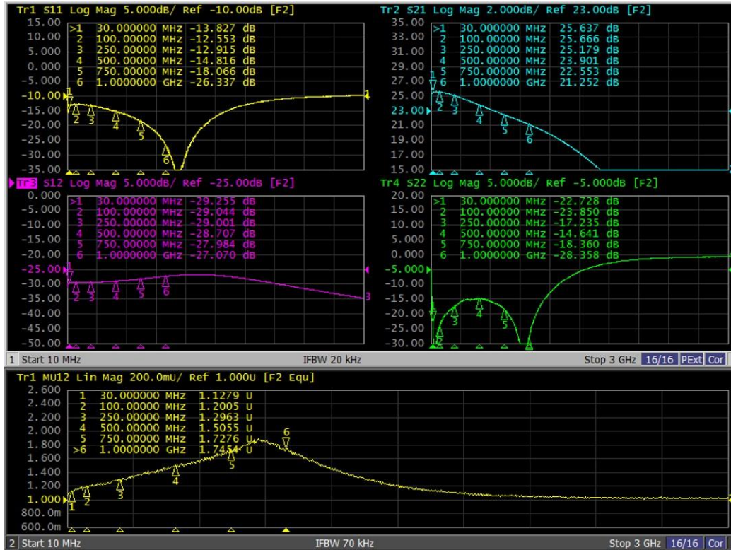
Figure 6.1.1. S parameters of TL0374J-EVB-C
