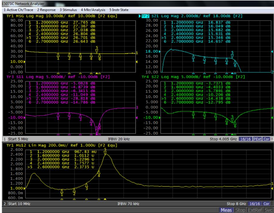
Figure 6.1.1. S parameters of TA9210D-EVB-H 28V 50mA
