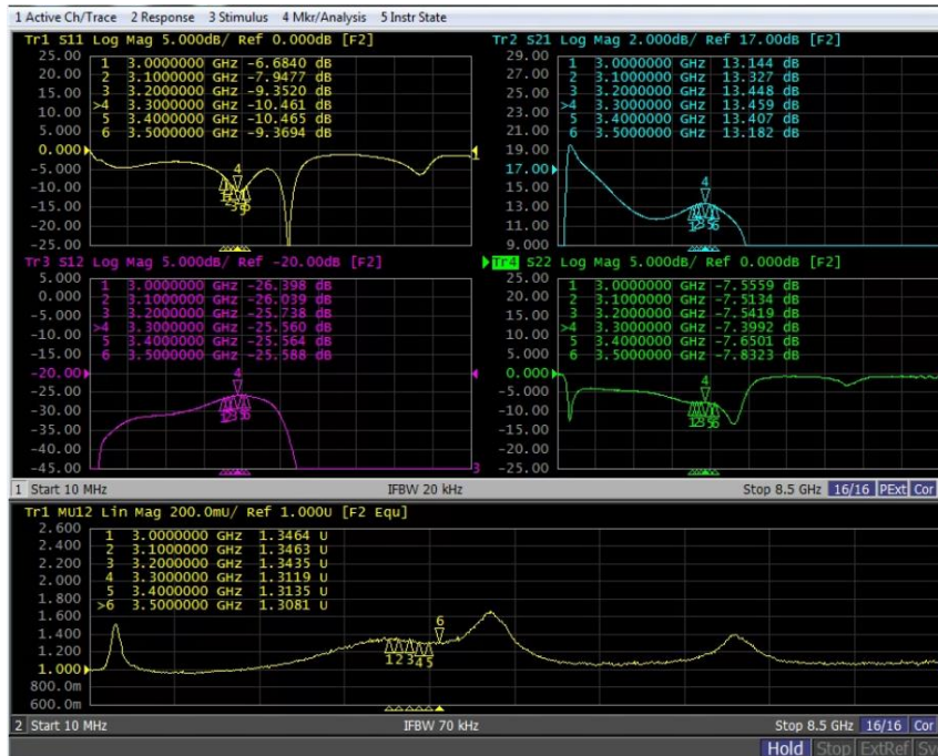
Figure 6.1.1. S parameters of TA9210D-EVB-J 24V 30mA
