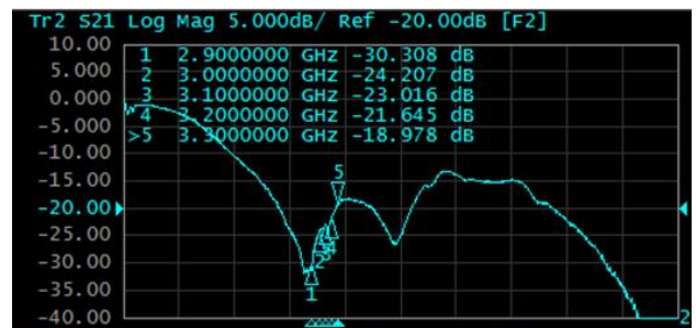
Figure 6.1.5. ANT to TX isolation of TSL8029N-EVB-E when RX-HG is on
