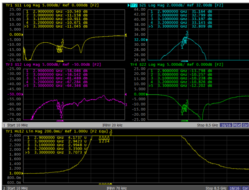
Figure 6.1.2. S parameters of TSL8029N-EVB-E RX-HG 5V 90mA
