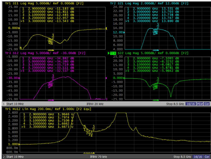
Figure 6.1.1. S parameters of TSL8029N-EVB-E RX-LG 5V 50mA
