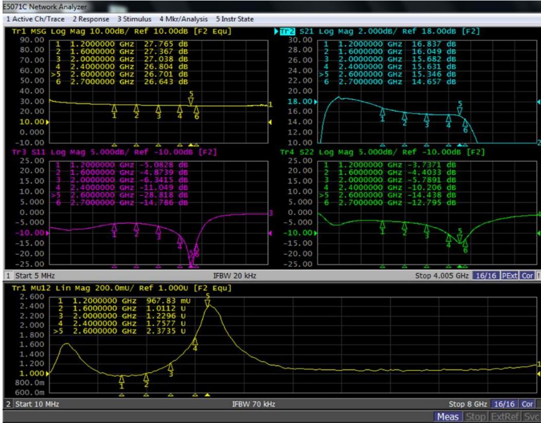
Figure 6.1.1. S parameters of TA9210D-EVB-H 28 V, 50 mA
