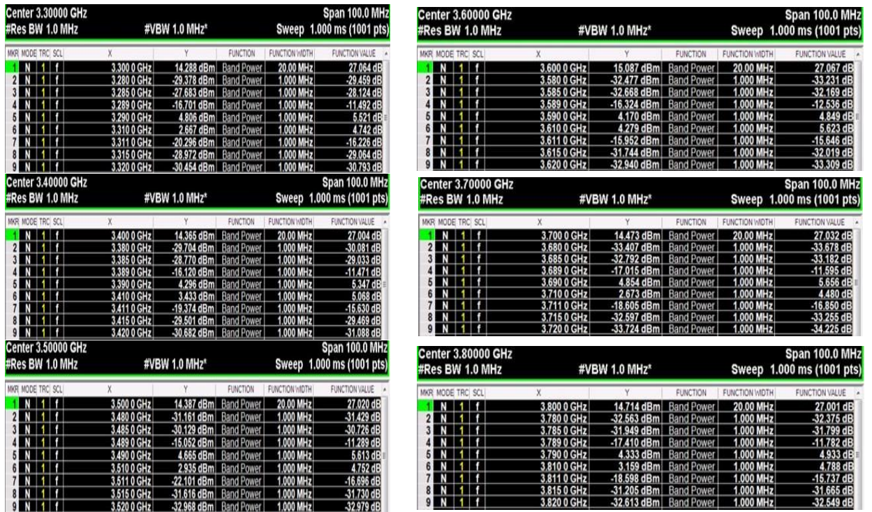
Figure 6.6.1. Spectrum Mask Plot @ Pout = 27 dBm, 36 V, 50 mA Idq
