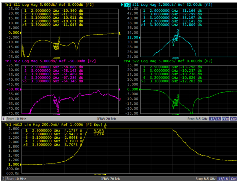
Figure 6.1.2. S parameters of TSL8029N-EVB-E RX-HG 5 V, 90 mA
