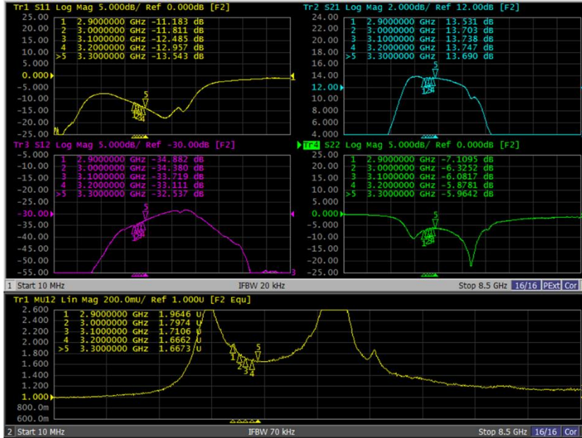
Figure 6.1.1. S parameters of TSL8029N-EVB-E RX-LG 5 V, 50 mA
