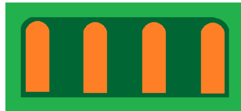
Figure 5.2 Solder Mask for < 0.5 mm Pitch Pins
