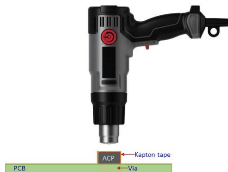
Figure 7.5 Manual Soldering Option 3
