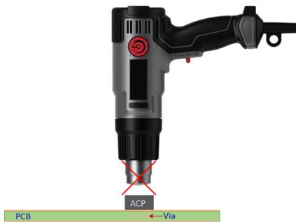
Figure 7.1 Prohibited Soldering Method
